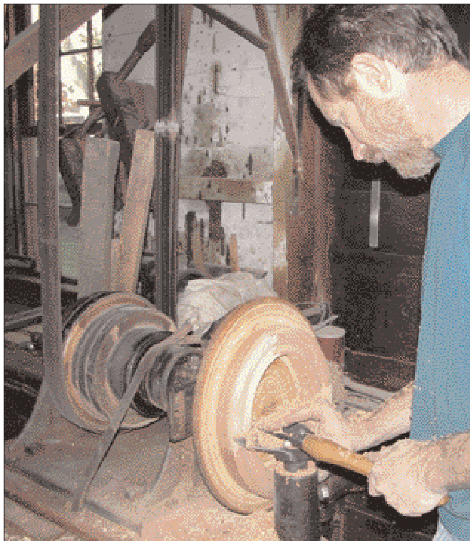
The mill's turner, David Graf, shapes the outside of a small oval frame. All steps—from raw stock through finger-jointing and turning—are performed at the mill. In the mill's historically accurate setting, eye protection isn't worn.
