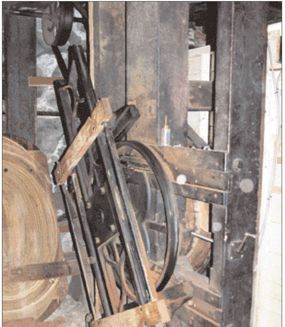
The frames produced on this lathe require a chuck almost 6½ feet across—and it moves several directions while turning. The middle of three posts is 12½" x 7".
