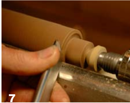
7 Remove the ferrule, then take light cuts with a skew to clean up the shoulder on the \frac{3}{4} "-wide tenon.
