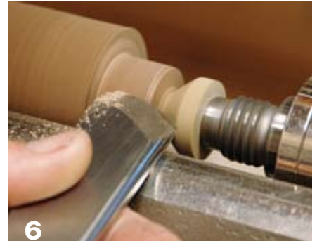
6 Use the skew as a scraper to size the tenon to match the diameter marked by the ferrule. Take light cuts and test the fit frequently.
