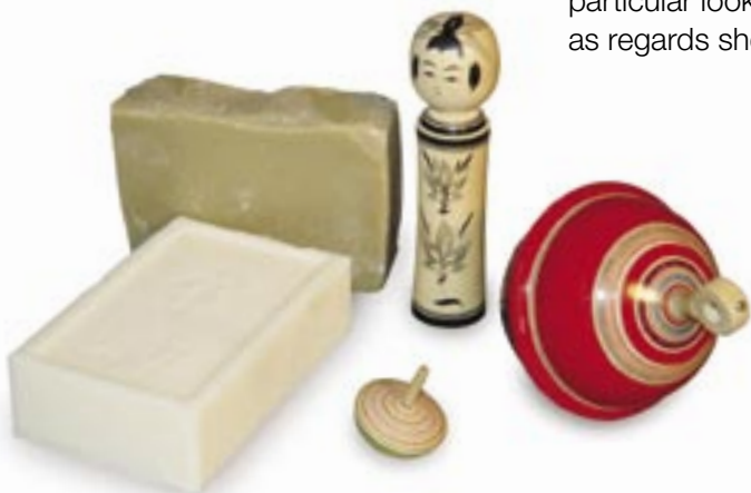
The Japanese toy, top, and kokeshi turners use wax almost exclusively. Their traditional wax, Japan wax, is not technically a wax but a vegetable tallow. However, it is applied and performs like anything we label as wax.
