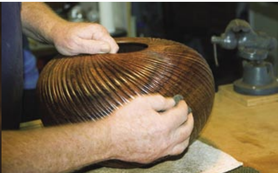
Apply stick wax to pieces while still mounted on the lathe. Bill Hunter softens the sheen of a cocobolo piece with 4/0 steel wool.
