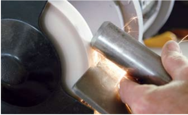
As a general guideline, high-carbon steel sparks remind some turners of sparklers. At the grinder, you should notice a complex shower of sparks.
