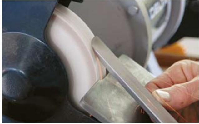
As a general guideline, high-speed steel (HSS) sparks remind some turners of tracer bullets and tend to be individual sparks. Note: This test is not always conclusive for HSS.
