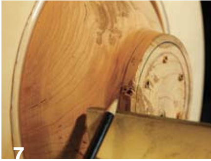
7 To center the piece on the chuck, use a pencil to find the high point of the bowl. Loosen the wing nuts, push from the center of the penciled length, and tighten the nuts.
