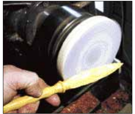
To shape the blade, the lathe becomes a sander. Mount a 5"-diameter plywood disc in a chuck or on a faceplate.
