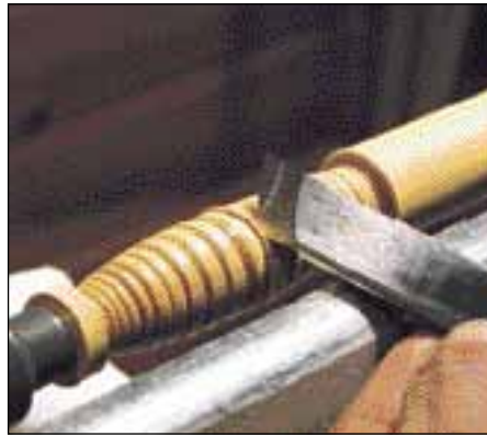
With a 1/2" skew, roll large beads with the short point and 1/4" or smaller beads with the long point.
