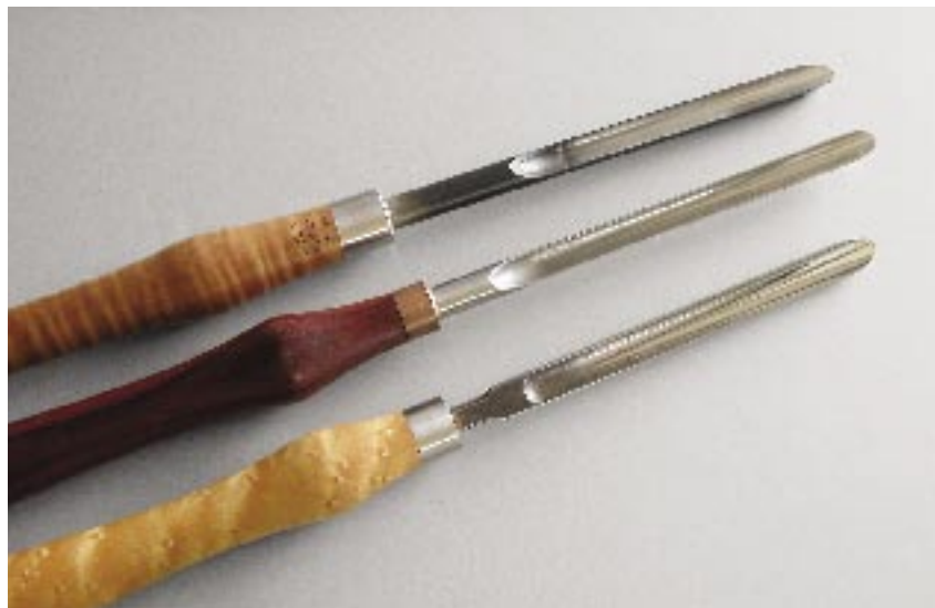
Right: Some of the earliest tools Jerry made in the 1960s for his friend Bob Stocksdale. The bottom prototype gouge was machined from rectangular bar stock.
