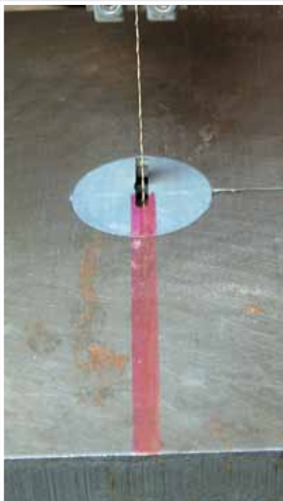
To crosscut short round stock, securing material in an adjustable parallel (handscrew) clamp is a solid solution.
